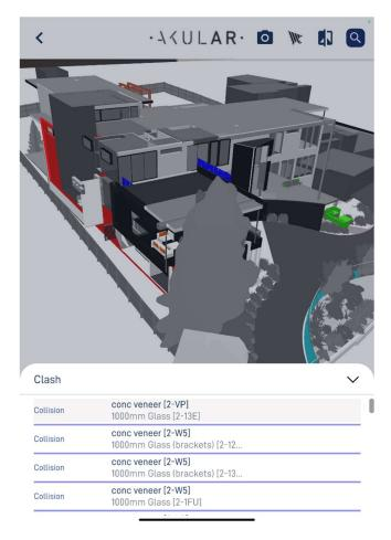
Caption: The powered by iTwin platform helps Akular users detect collisions and check the clearance between geometric elements.
